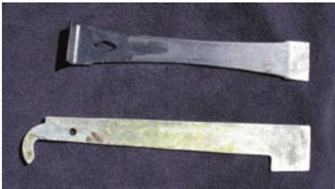
Figure 17. Standard hive tool on top. Maxant tool on bottom
